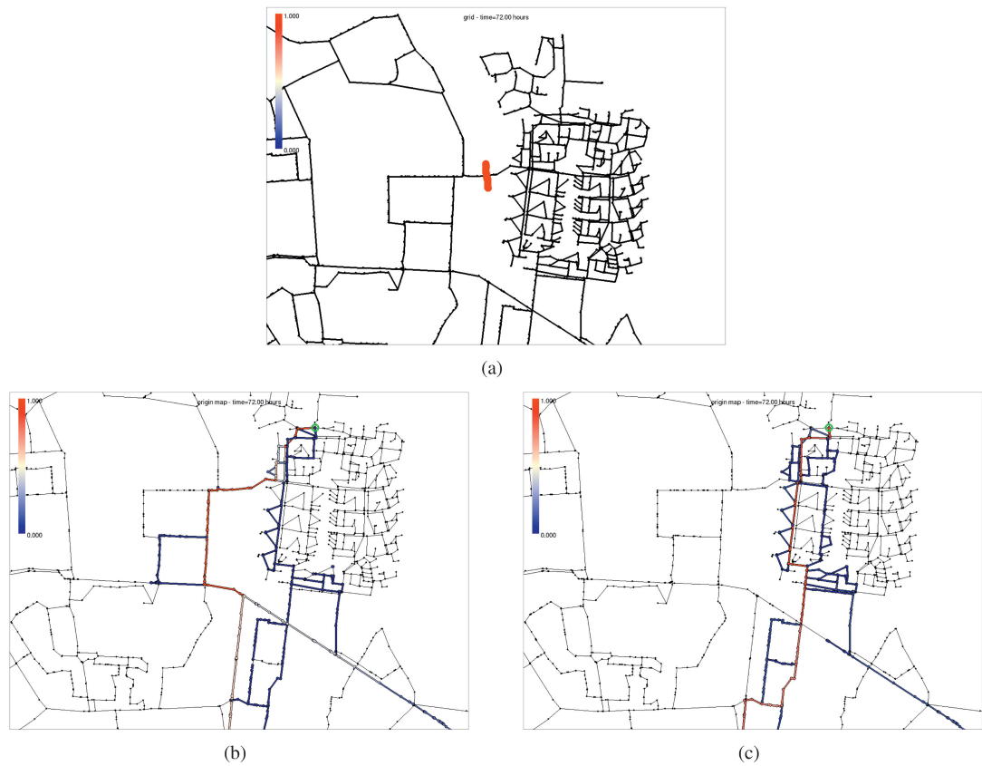
Fig. 6. The closing of a single valve (a) leads to a complete change in the origin map (b to c) for a node which is close to this valve.
