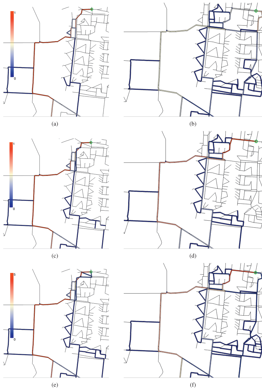
Fig. 4. Origin maps for water sampled at two marked locations (a,c,f and b,d,f) at time t=72 hours for two different realisations of the flow field (a,c and b,d, respectively) with combined maps for 5 realisations (e,f).
